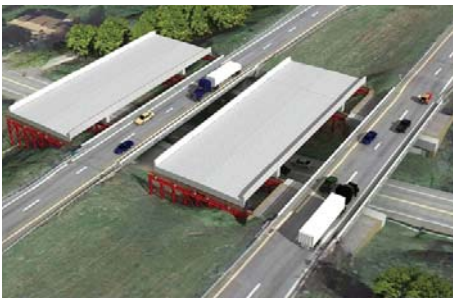
Step 1: Construct superstructure next to existing bridges
